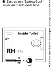
When standing looking into the cavity pocket, if the locking snib is on your *right hand* side then the LaviLock is a Right Hand lock.
