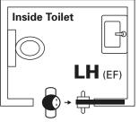
When standing looking into the cavity pocket, if the locking snib is on your left hand side then the LaviLock is a Left Hand lock.
